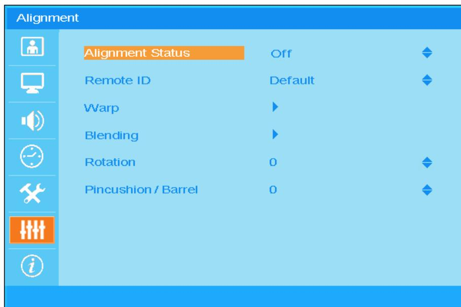
7. Projector Setup 4 : Enter **Warp** and fine tune the screens by the Warp functions
